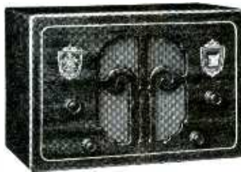
MODEL 355 —(Left for A. C.—D. C. Current) and MODEL 350 (Right for A.C. Current)—5 tube, 8 tube performance Dual Wave, Vibro-Power superheterodyne Personal Radio. Portable. Size 11 3/4" wide x 7 7/8" high x 6 15/16" deep. Built-in antenna. Range 530 to 4200 Kilocycles (368 communication channels). Full automatic vol-
